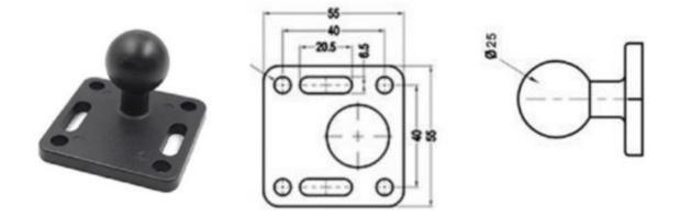
The device will be attached to a 1 inch ball head as shown in the picture above. This ball mount must be attached to the vehicle with tight screws at a location as described above. The diameter of the screw holes is 6.5mm and the distance between the holes is 40mm. When mounting on the dashboard, a support plate must be attached to the back to prevent the screws from breaking through the plate in the event of an accident to prevent the holder from flying around freely in the vehicle.
